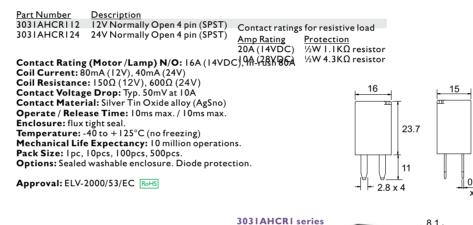
3031AHCRI series 85 **Terminal Size** \_\_\_\_\_ 🖵 2.8mm  $\sim$  $\mathcal{M}$
