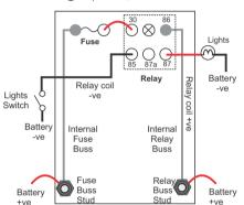
RTMR Block with 2 Input Studs
