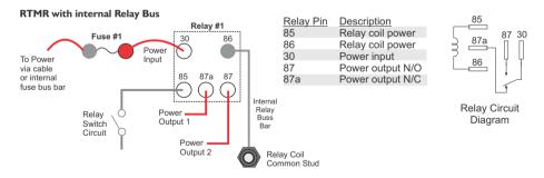
As you can see in the above illustration, relay coil pin 86 is connected to the internal relay bus bar. Relay common pin 30 is connected to a fuse on the RTMR block using a jumper cable. Depending on how you wish to switch the relays, the relay coil stud can be connected to either positive or ground. However, if the relay is diode protected, it can only be wired in one configuration that will be determined by the polarity of the diode.
