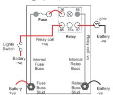
RTMR Block with 2 Input Studs
